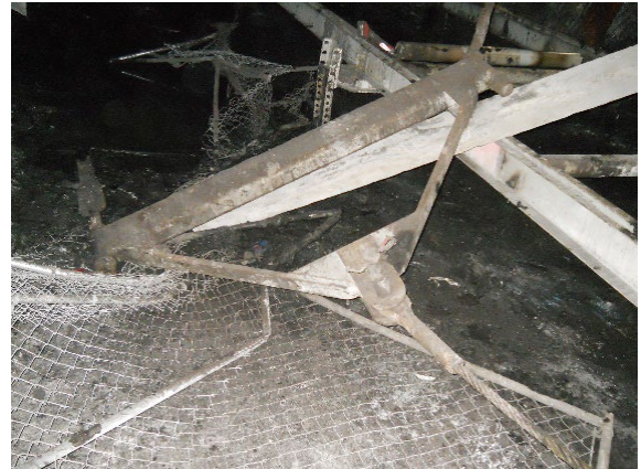
A belt foreman was fatally injured when a longwall belt conveyor take-up unit component, the bridle, broke and struck him.
